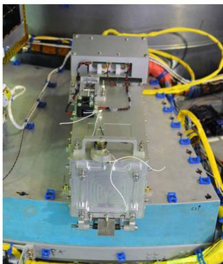
Figure 29: IIT Kanpur Deployer system on the upper stage.
