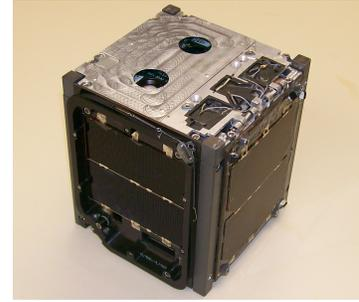
Figure 4: CP6, showing the deployable top panel [11].
