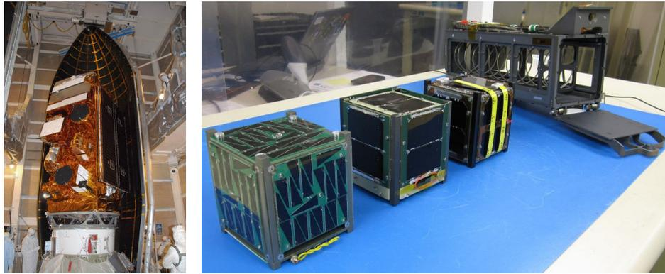
(a) NPP, with the P-PODs mounted in the lower right. (b) AubieSat-1, HRBE, and M-Cubed before integration.
