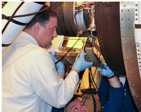
Figure 28: P-POD being mounted to the aft end of the Taurus XL [74].
