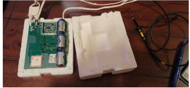
Partially-disassembled LMS-6 Radiosonde, with upper styrofoam shell removed. Some RF shielding removed. Rechargeable cells in use for testing purposes.
