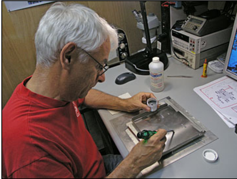
Photo 10. I Apply the Solder Paste
