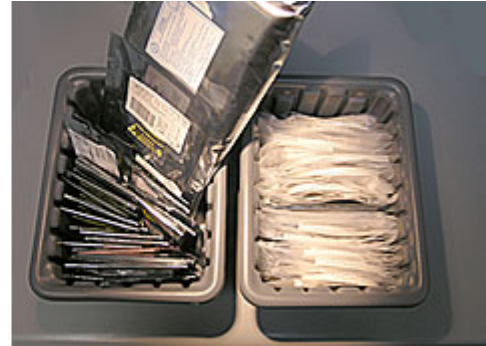
Photo 8. Three-Inch binder and ESD parts bins sorted by reference designation
