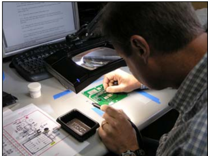
Photo 11. Greg Places Components on the PCB
