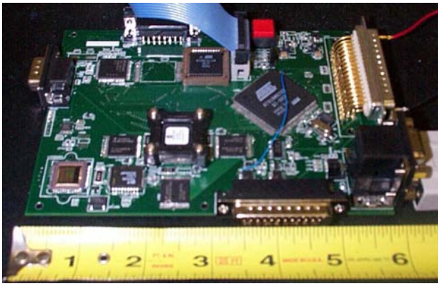
Fig. 6. CanX-2 Prototype On-Board Computer. Note that smaller connectors will be used on the flight-ready OBC.
