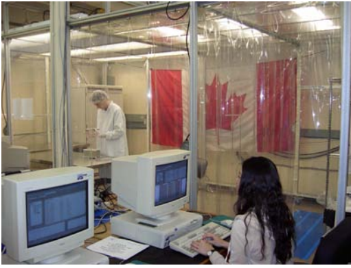
Fig. 2. Class 10,000 Clean Room Facility at UTIAS/SFL.
