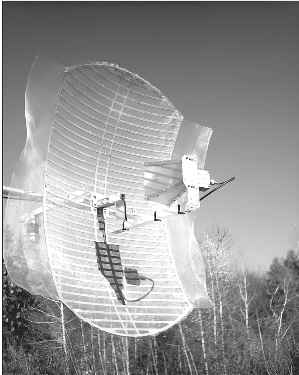
Figure 16. Completed dish antenna with horn feed
