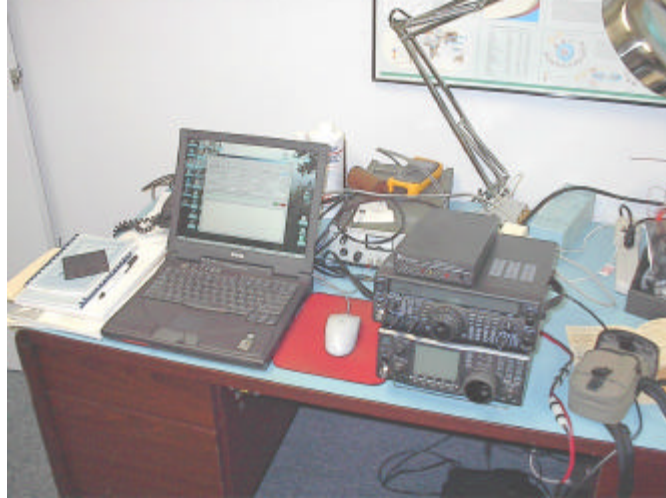
Figure 11 – RF Test Setup during Integration at SpaceQuest
