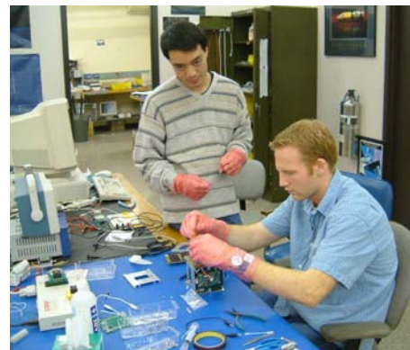
Fig. 1. Master's students get hands-on training by assembling CanX-1 on the lab bench.
