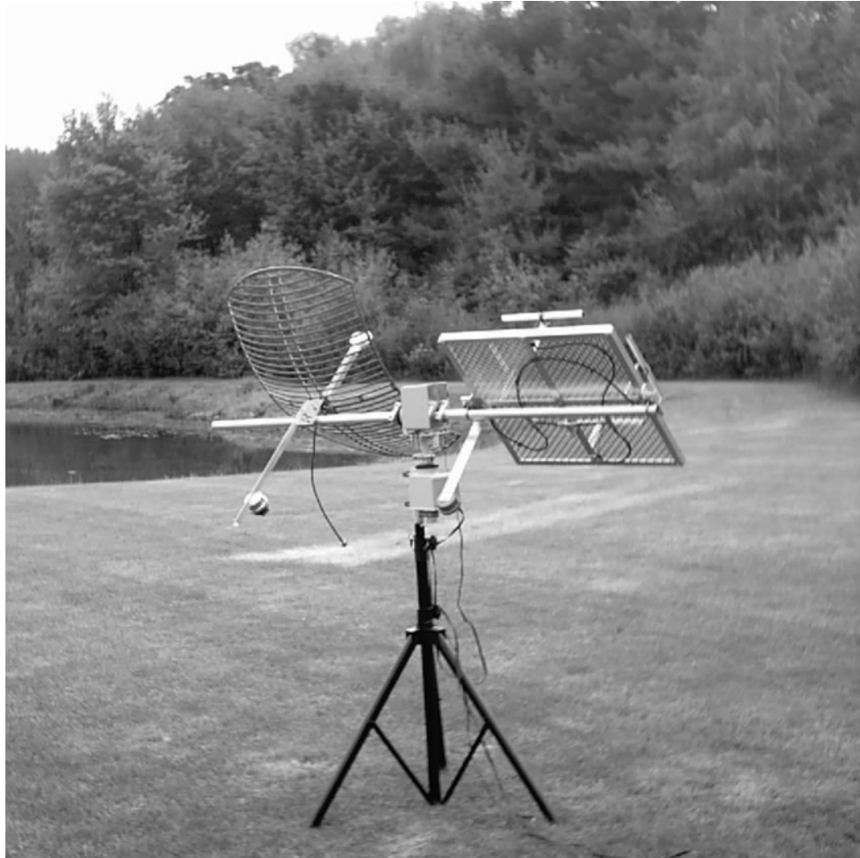
Figure 2. Test azimuth/elevation positioner made from TV antenna rotators
