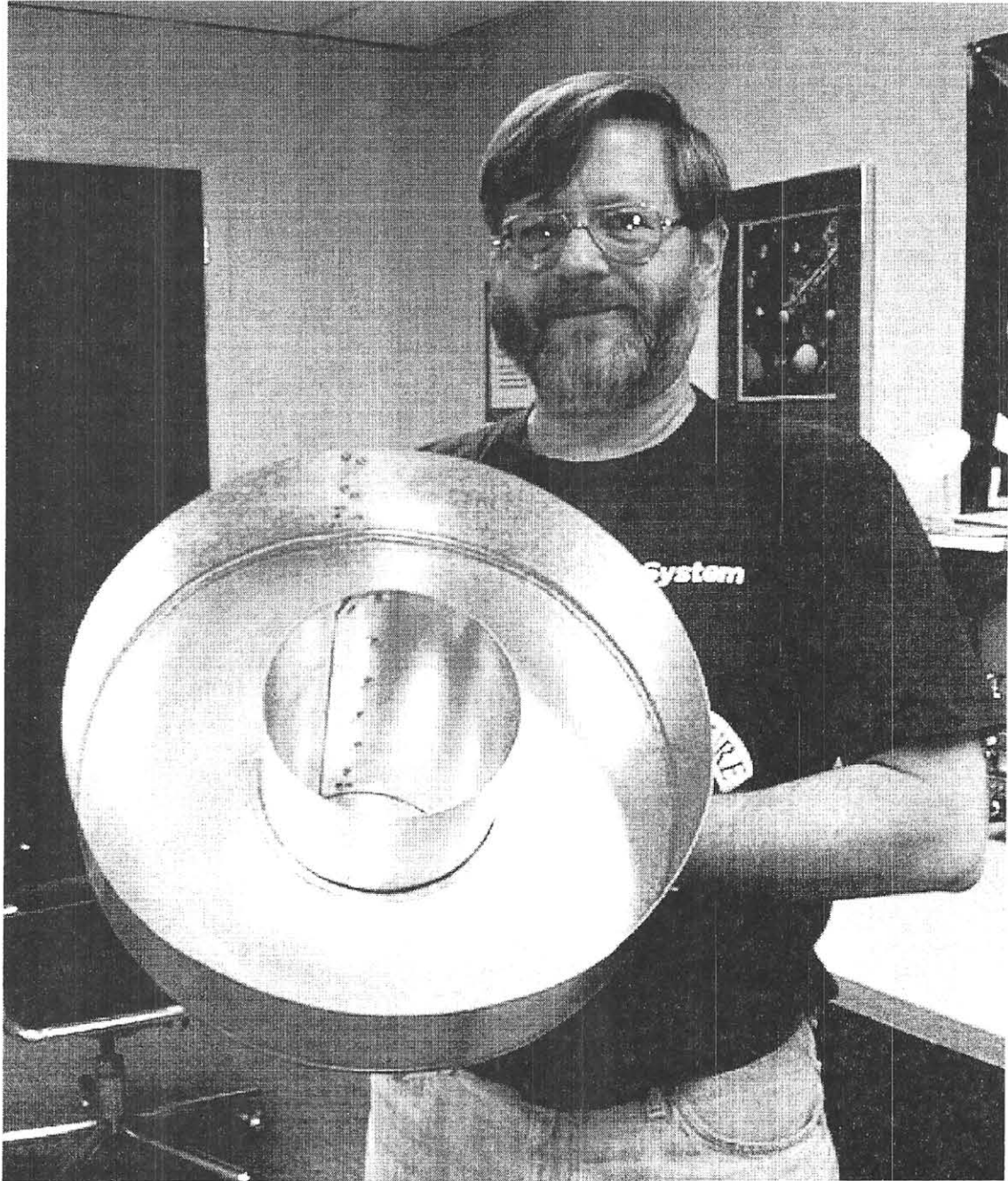
Figure 3 N6TX with Radio Astronomy Supplies feedhorn for the 1420 MHz SETI band
