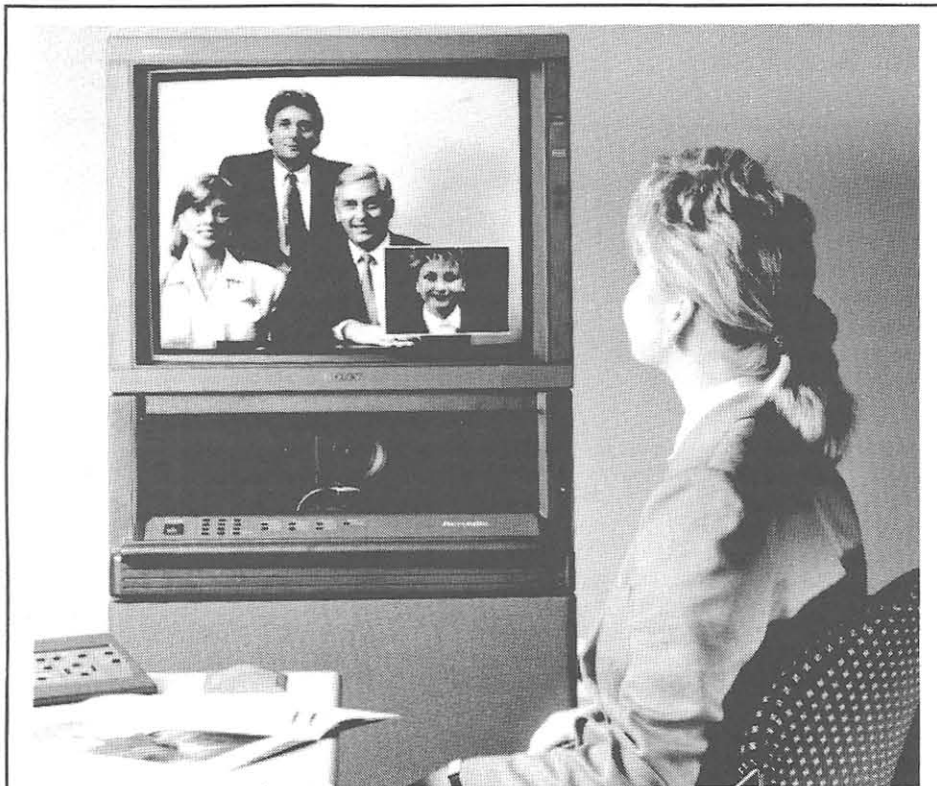
PictureTel Corporation's video conferencing systems make two-way digital video communications possible over special dial-up digital phone lines (two "Switched 56" Kbps circuits = 112 Kbps total bandwidth). The system is based on a specialized computer called a codec (coder/decoder) which does the digitalization of the video and audio and then compresses the signal. (PictureTel Corporation photo)
