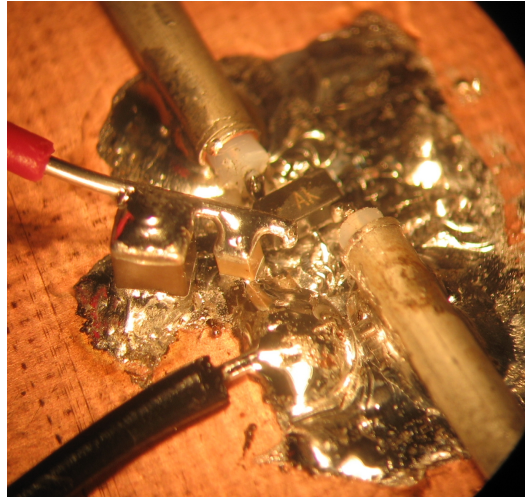
Figure 8: Oblique picture of the LNA test fixture. The 10\mu\text{F} bypass capacitor, at left, is bigger than the 1\mu\text{F} bypass capacitor. This chip is upside-down, so RF Input is from the top, and output is toward the bottom.
