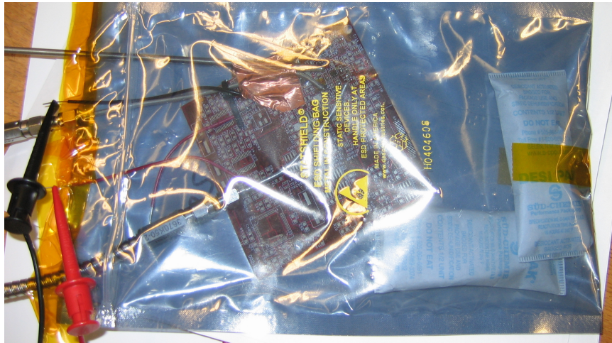
Figure 21: Set-up for the thermal testing. The desiccant bags on the right prevents condensation from shorting out the chip. The temperature probe is under the copper tape at the top.
