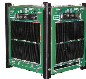
Figure 22: CAPE1. The turnstile antenna doors are visible above the solar cells.
