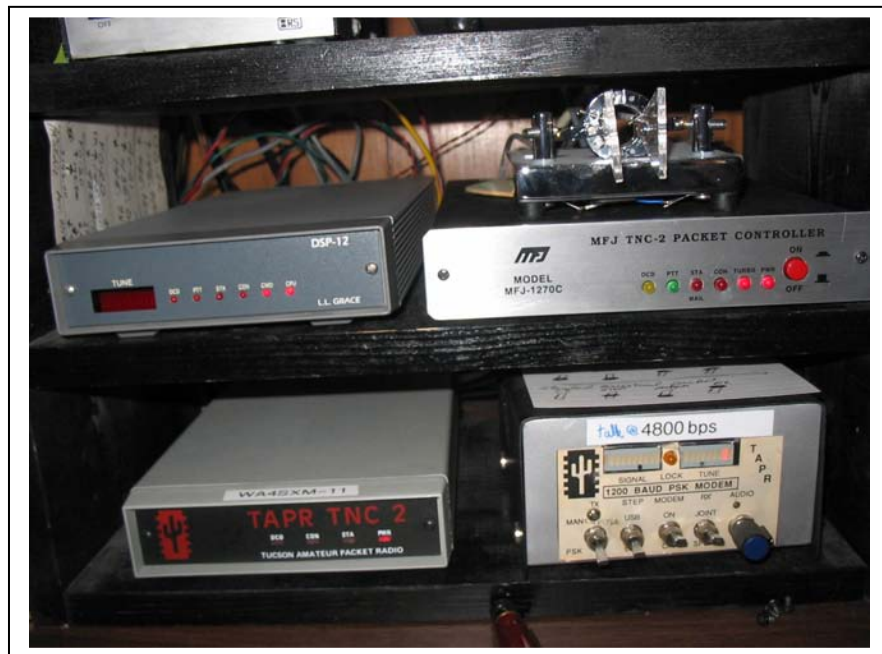
Figure 7. A host of satellite modems, lower right CCW - 1200 bps PSK modem addition to TNC 2, a 9600 bps FSK modified TNC 2 and DSP-12 modem.
