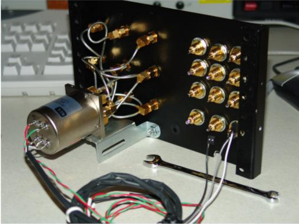
Rear Panel Showing PTT and Control RCA Jacks
