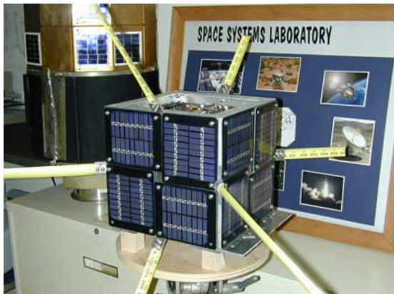
Photo 2. Prototype Communications Satellite (PCsat) with Antennas
