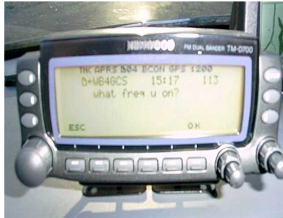
Photo 9. The front panel of the TM-D700 showing an incoming 15 byte message (Messages can be up to 64 bytes).
