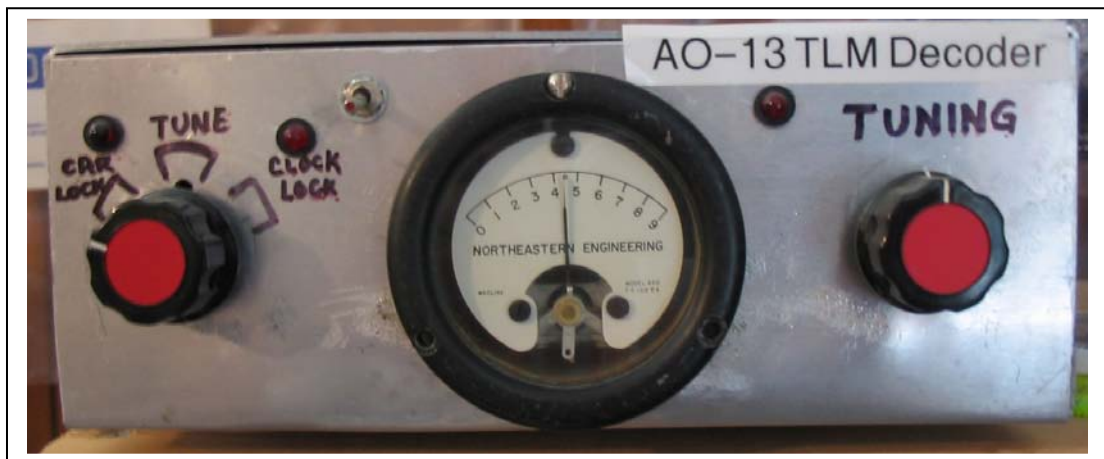
Figure 10. Yet another telemetry modem, 400 bps G3RUH modem for Phase 3 telemetry
