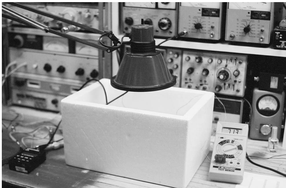
Figure 11. Testing the XP217 models at +40C
